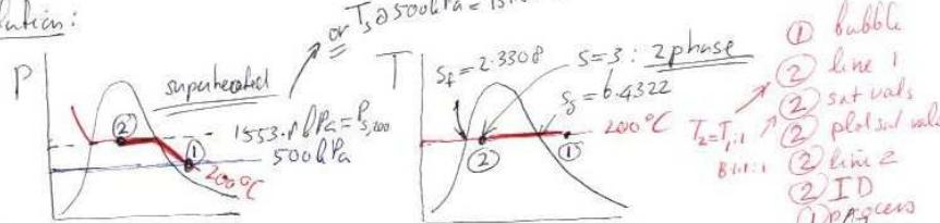
② Table B-1.3 at 500 kPa, 200°C :  $h_1 = 2855.37 \frac{\text{kJ}}{\text{kg}}$ ,  $s_1 = 7.0592 \frac{\text{kJ}}{\text{kg}\cdot\text{K}}$
