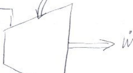
$$\text{1st law } \dot{Q} + \dot{m}(h_i + \frac{1}{2}V_i^2 + gz_i) = \dot{W} + \dot{m}(h_e + \frac{1}{2}V_e^2 + gz_e)$$
