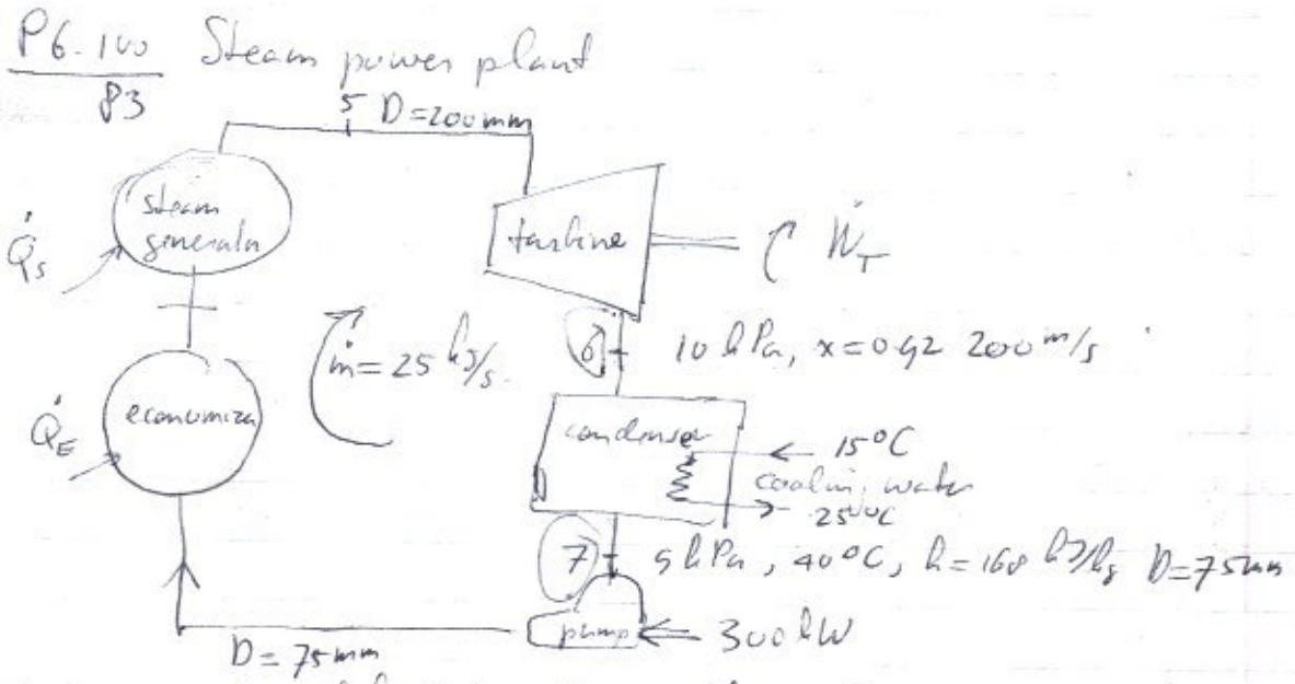
Asked: rate of heat transfer in the condenser, and the mass flow rate of cooling water.
