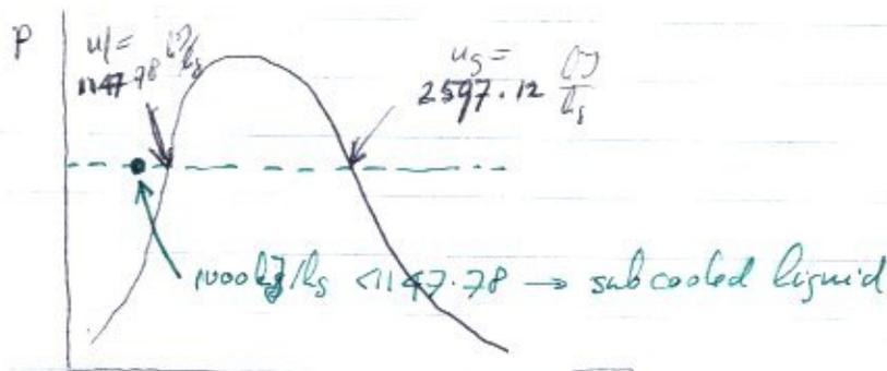
Table B.1.4 <sup>A7</sup> compressed liquid water  $p = 600 \text{ MPa}$  @  $5000 \text{ Pa}$  @  $u = 1000 \frac{\text{J}}{\text{kg}}$
