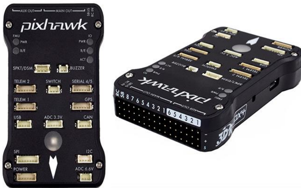
Figure 8 - Flight control hardware - Pixhawk [2]
