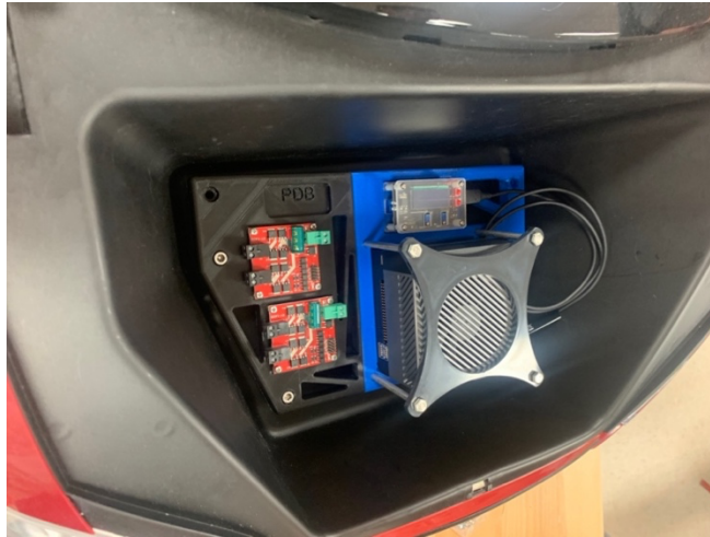
FIGURE 13: NVIDIA JETSON IN FRUNK
