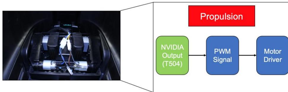
Figure 8: Propulsion Subsystem
