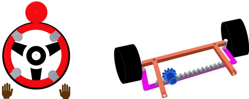
Figure 5: Initial v. Final Steering Designs
