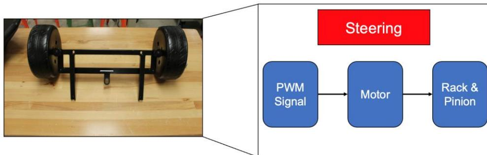
Figure 4: Steering Subsystem
