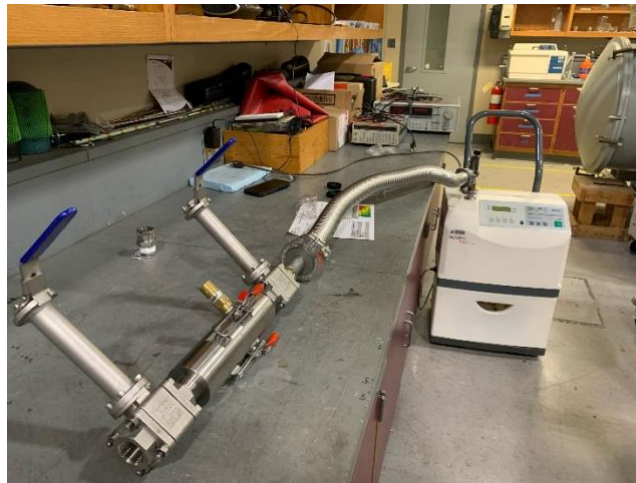
Figure 3 Leakage Test Experimental Setup
