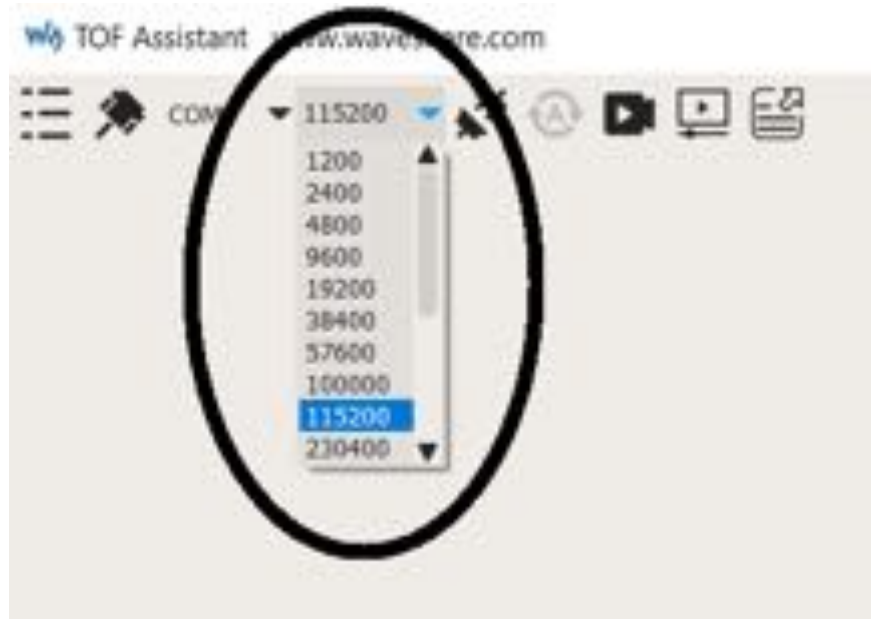
Figure 17: Changing the Baud Rate on the TOFAssistant Software
