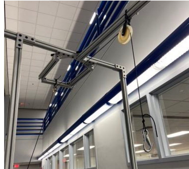
Pulley to Lift Lander
