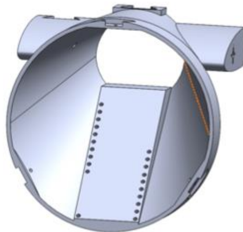
Figure 15. Location of the box weight inside the fuselage.
