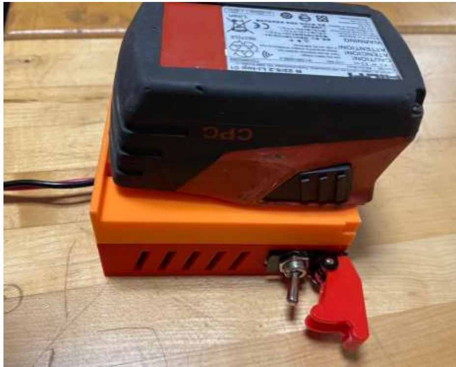
Figure 7 Assembly of battery system.
