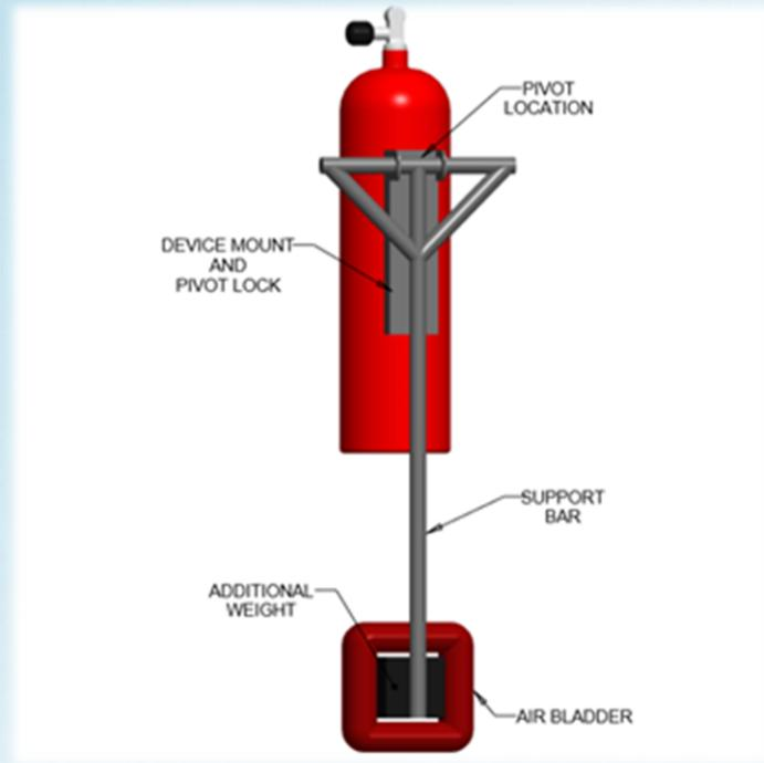
Secondary Buoyancy Compensator
