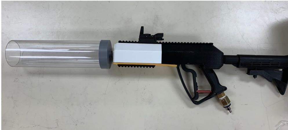
The net launcher is the most important component for neutralizing the drone it consists of the PLA frame that holds the components together mounted to this frame are picatinny rails to support various attachments, the trigger system, an ergonomic stock to improve accuracy, and the net holder
