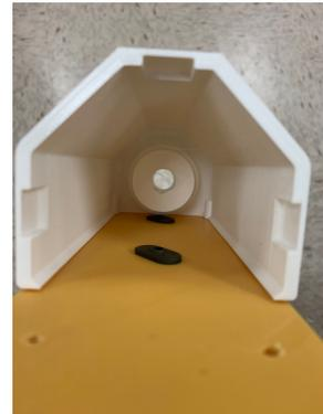
The lower plate is then connected to both prints using the 0.125” screws provided. There are four screw locations, two on each print.
