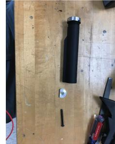
Once the tube is attached to the print, the stock is ready to be connected. To connect the stock simply push down on the back of the tab located under the stock frame, and slide the stock down the buffer tube.
