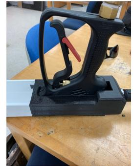
Once snug, the trigger assembly can be secured to the prints by attaching the lower plate that is assembled in the next step.
