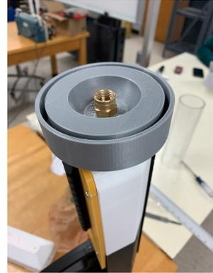
Lastly, attach the tubing that the net is placed inside by pushing it down into the adapter.
