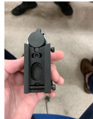
With the screws loosened, place the sight onto the rail and rock back and forth until the screws slide and is caught by the rail. Tighten the two screws using the 3/32" allen key.
