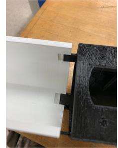
Once the prints are secured together by the tabs, screw in the top rail to the back print to secure the two prints.
