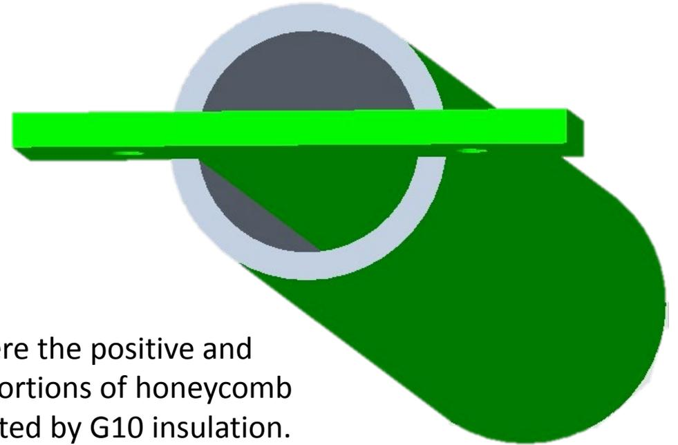
As seen here the positive and negative portions of honeycomb are separated by G10 insulation.
