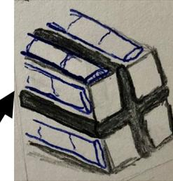
Exploded view of HTS-laced Copper leads
