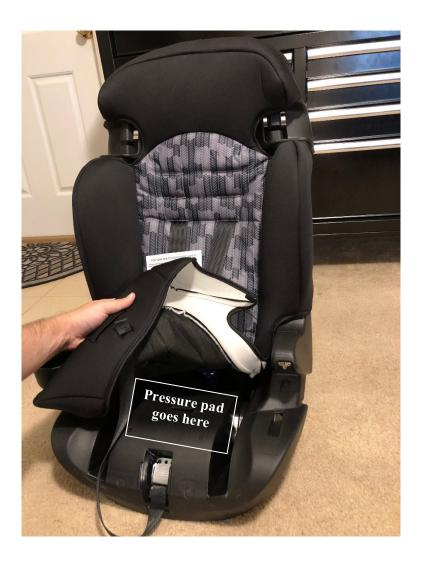
After attaching the vehicle module to the car seat, lift the car seat cushion liner and slide the pressure pad in between the cushion and the plastic of the car seat. Ensure that the pressure pad is centered on the seat and does not crease while performing this procedure. Route the pressure pad wire around to the vehicle module and connect the wire. Push firmly until the connectors are locked together. Make sure to secure any loose wires.
