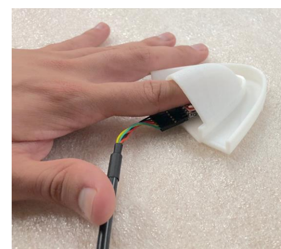
Figure 2.0 - Actual printed mouthpiece casing. Casing size based on MRI Scan of oral cavity. Used as a light blocking shield for the sensor-controller unit for testing purposes
