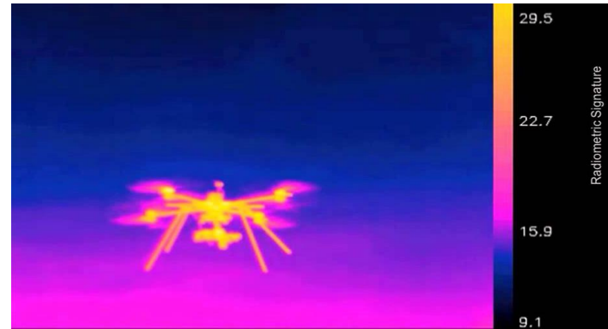
Figure 6: drone detected on thermal imaging [2].
