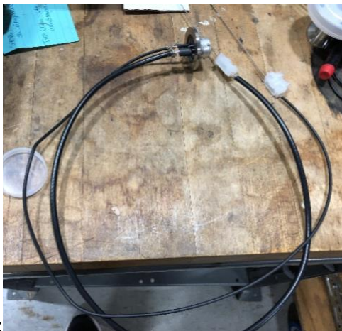
Figure 2: Tungsten Rod with Wire Configuration
