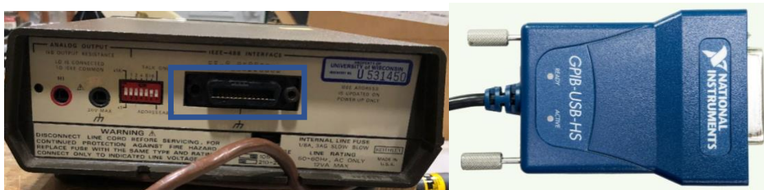
Figure 7: Back of the Voltmeter GBIB Connection
