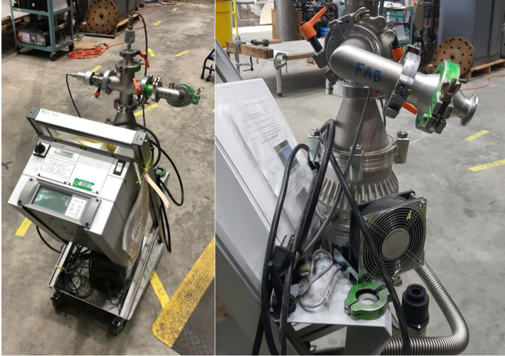
Figure 7: Vacuum/Diffuser Pump System with Gauge Controller
