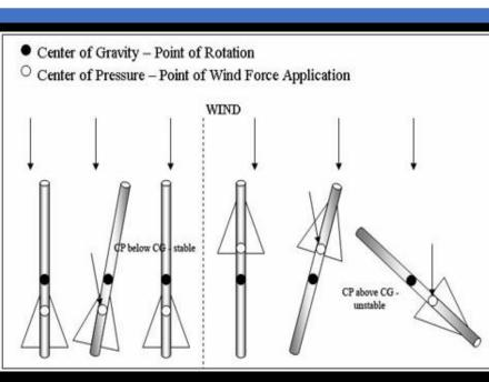
Figure 1. Location of Center of Gravity and Pressure Affect Stability
