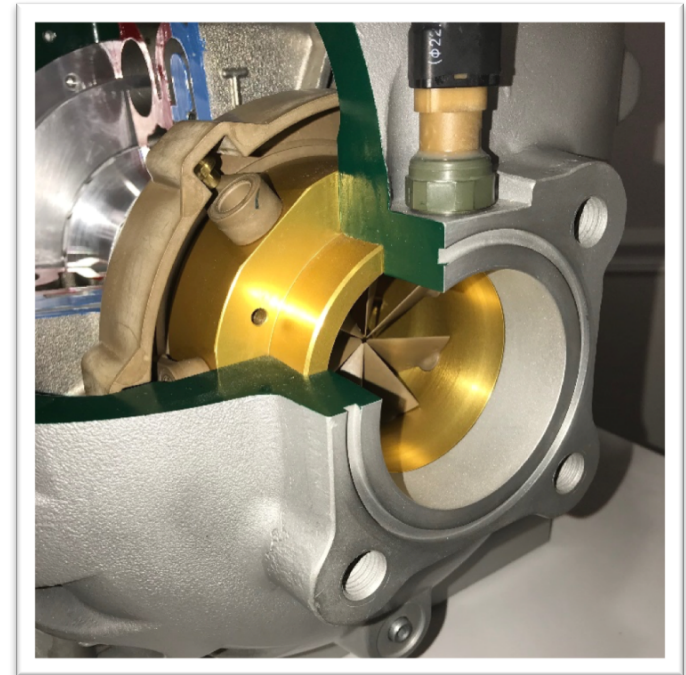
Compressor Inlet Cutout
