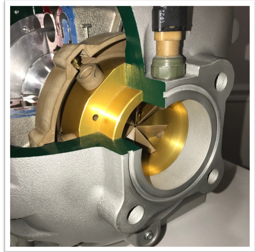
Compressor inlet cross-section with IGV detail
