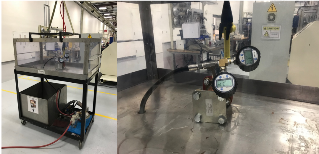
Figure 22 Pressure Burst Test Setup.
