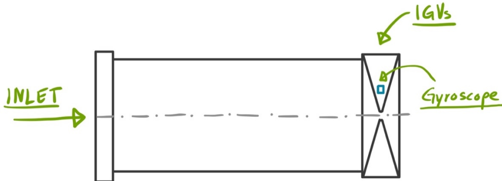
Figure 11. Angle monitoring concept utilizing a gyroscope.
