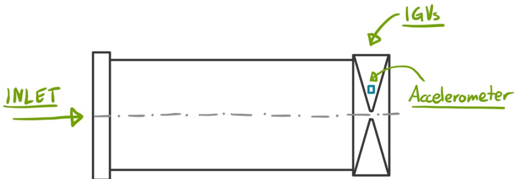
Figure 7. High cycle monitoring concept utilizing an accelerometer.
