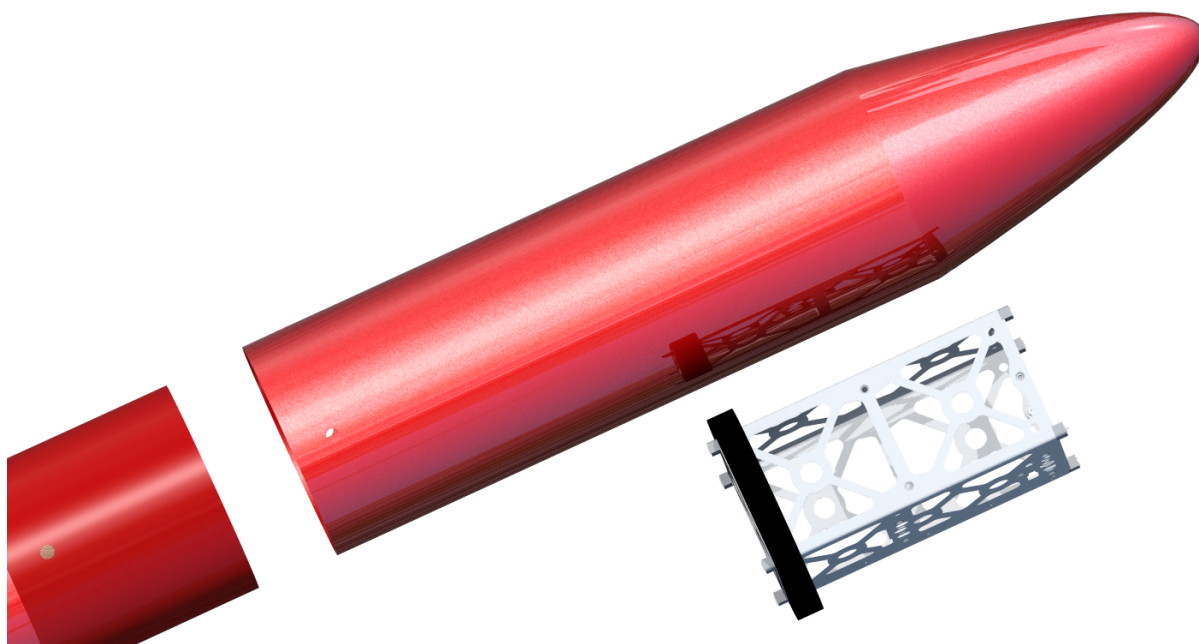
Figure 28: The payload will be housed inside of the nose cone and attached tube section.
