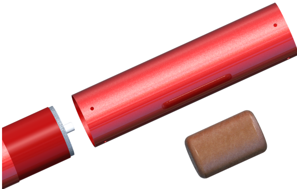
Figure 24: The drogue bay shown immediately following the booster section. In this section the parachute is represented by a brown cylinder and the kevlar shock cord is not shown to increase view-ability.
