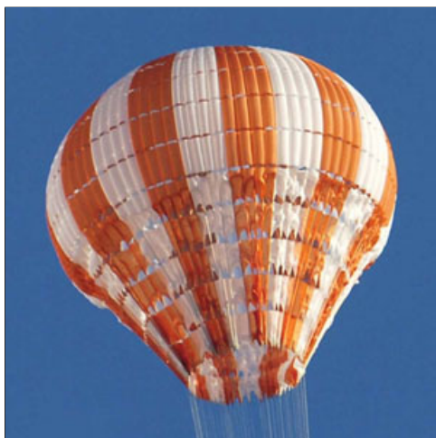
Figure 11: A large-scale reefed parachute system after deployment, still in its reefed stage. [9]
