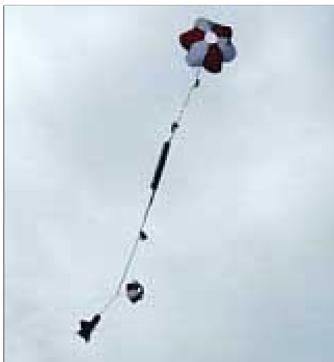
Figure 10: A dual deployment parachute system after deployment. [7]
