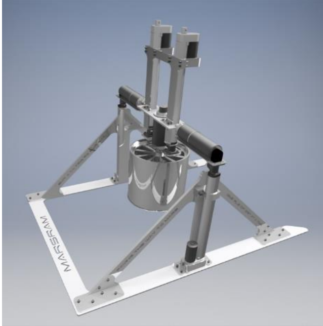
Figure 30: Isometric View of Mining Rig.
