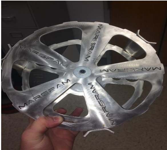
Figure 23: Manufactured Wheel, Based on CAD.
