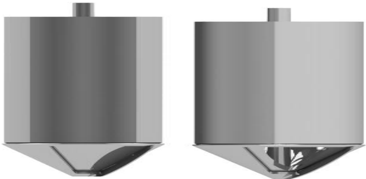
Figure 33: CAD of Mining Bucket Design (Open and Closed configurations).
