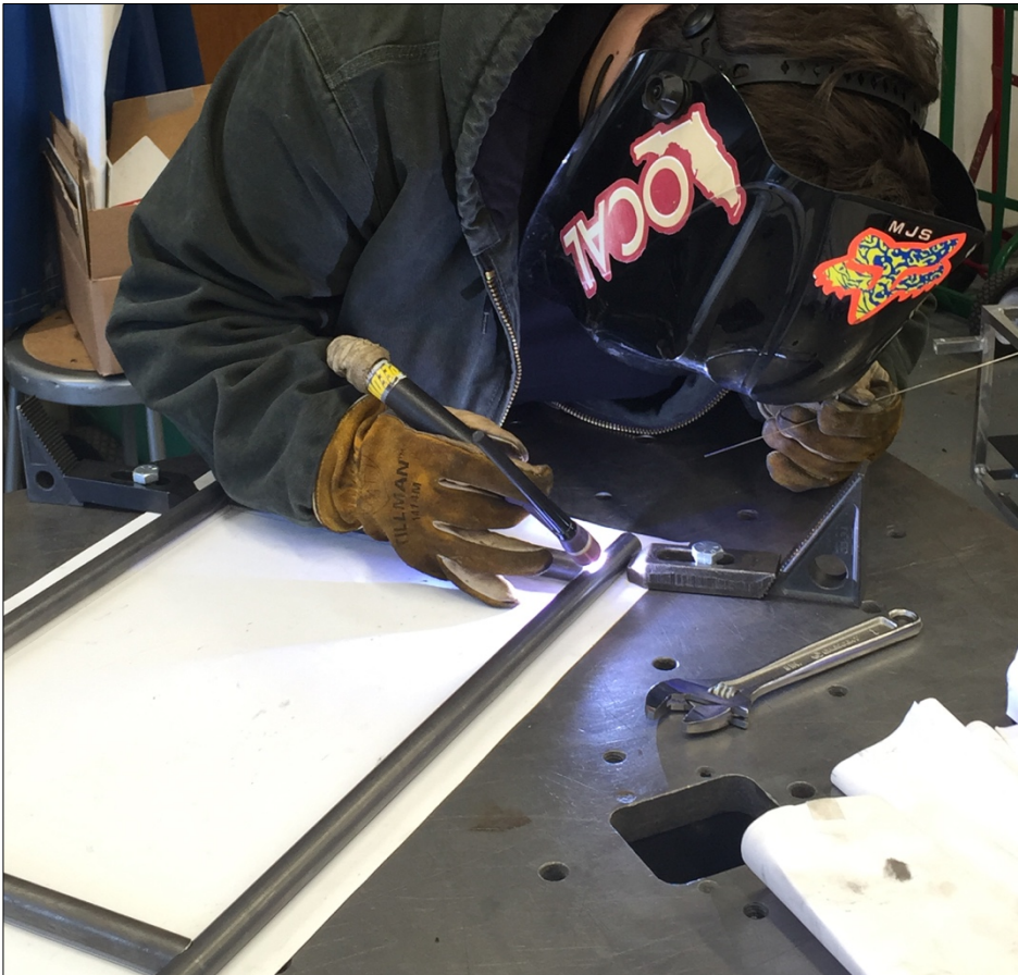
Figure 4. Machine shop employee welding the frame
