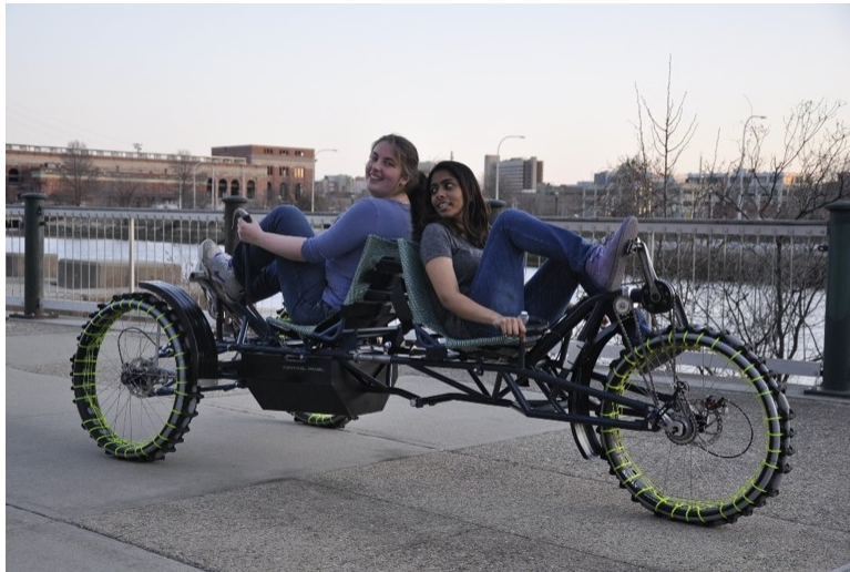
Figure 15: RISD Back to back configuration [3]
