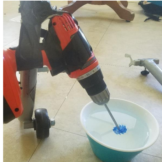
Figure 14 Electric drill being used to create a current
