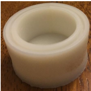
Figure 11 HIPS bottom mold
