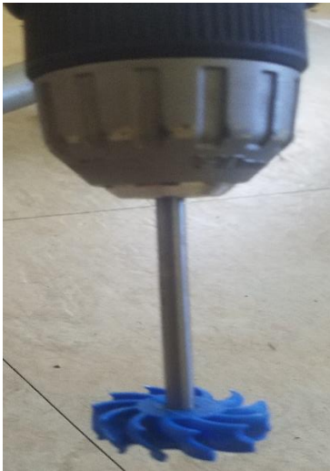
Figure 13 3D printed mixing propeller in bath
