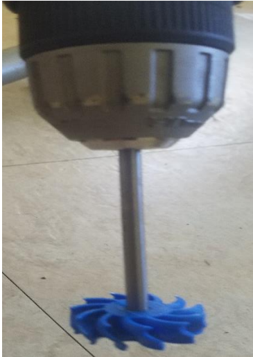
Figure 4 3D printed mixing propeller current in bath
