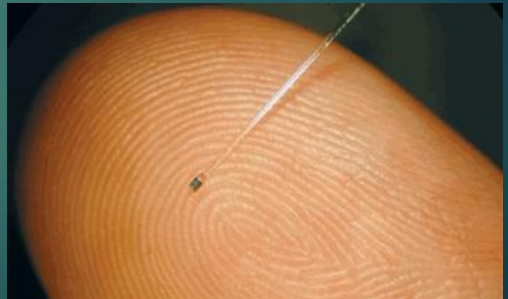
Figure 4 Displays the size of a fiber optics pressure sensor
