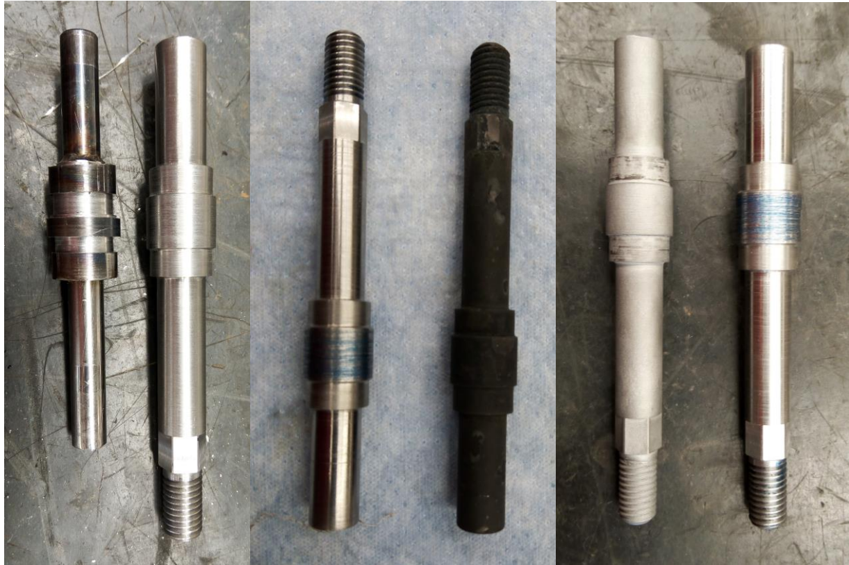
Figure 13: Original shaft vs new shaft (left), before and after heat treatment (middle), before and after the heat treated shaft was cleaned up (right).
