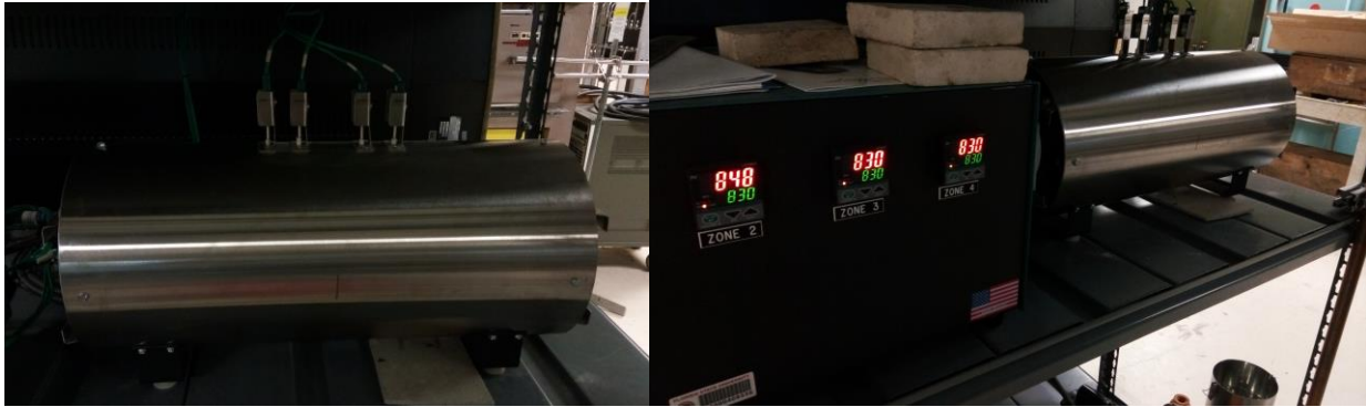
Figure 14: On the left is the furnace that was used and on the right is the power supply with the temperatures of each zone and the furnace.
