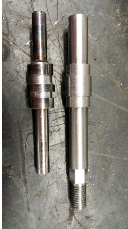
Figure 10: Original shaft (left) redesigned shaft (right)
