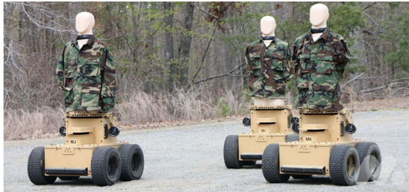
Figure 3: Robotic dummy with integrated fall-down mechanism upon “fatal” ballistic impacts [4].
