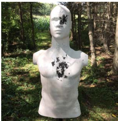
Figure 1: Rubber dummy with impact indication [2].
