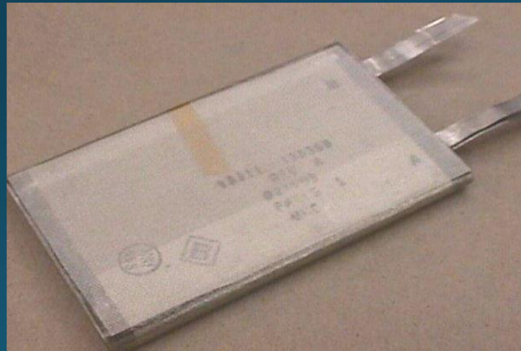
Figure 3: Individual Capacitor 2.6" x 4.25"
