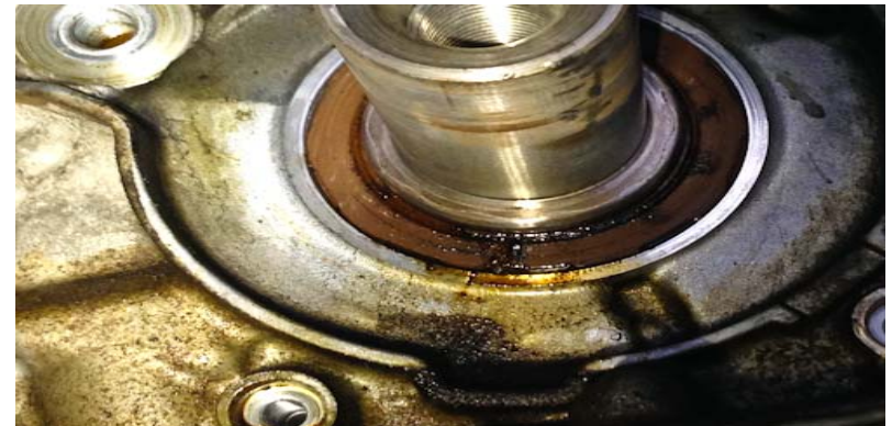
Figure 1: Depiction of rear crank seal leaking oil. 2
