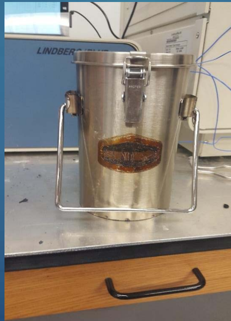
Dewar Flask after the fire test
