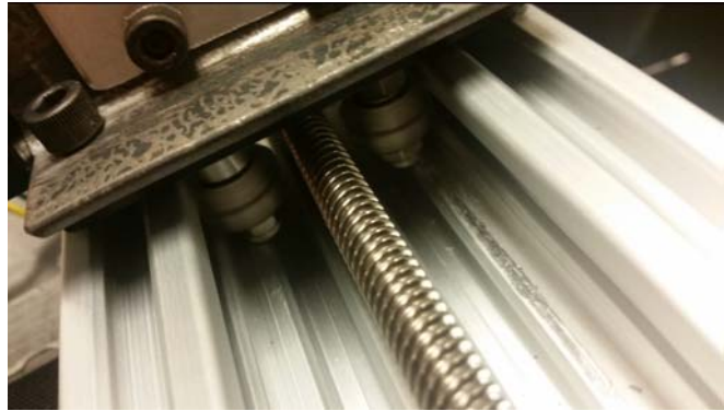
Figure 19: Contact between Wheel and Guide Rail
