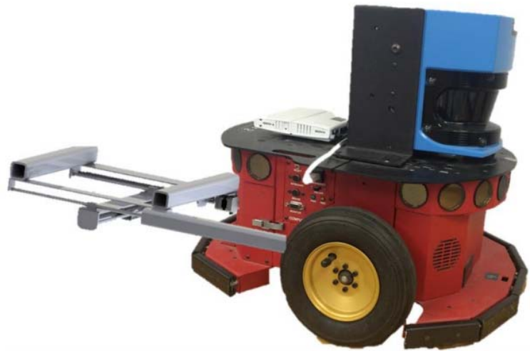
Figure 13: Mounting of Gantry System
