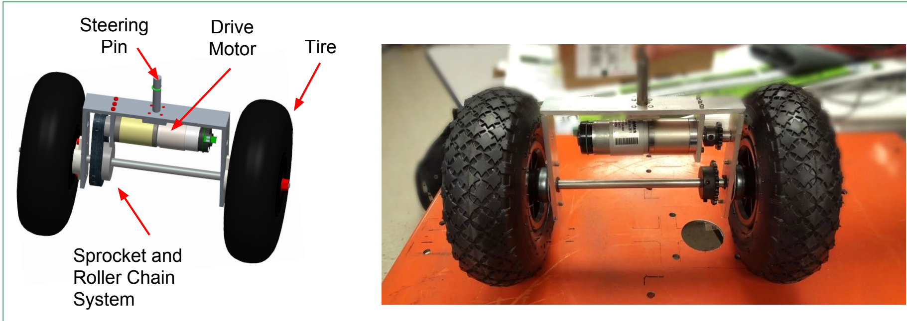
Figure 6: Steering and Drive Assembly; CAD to Actual Component.
