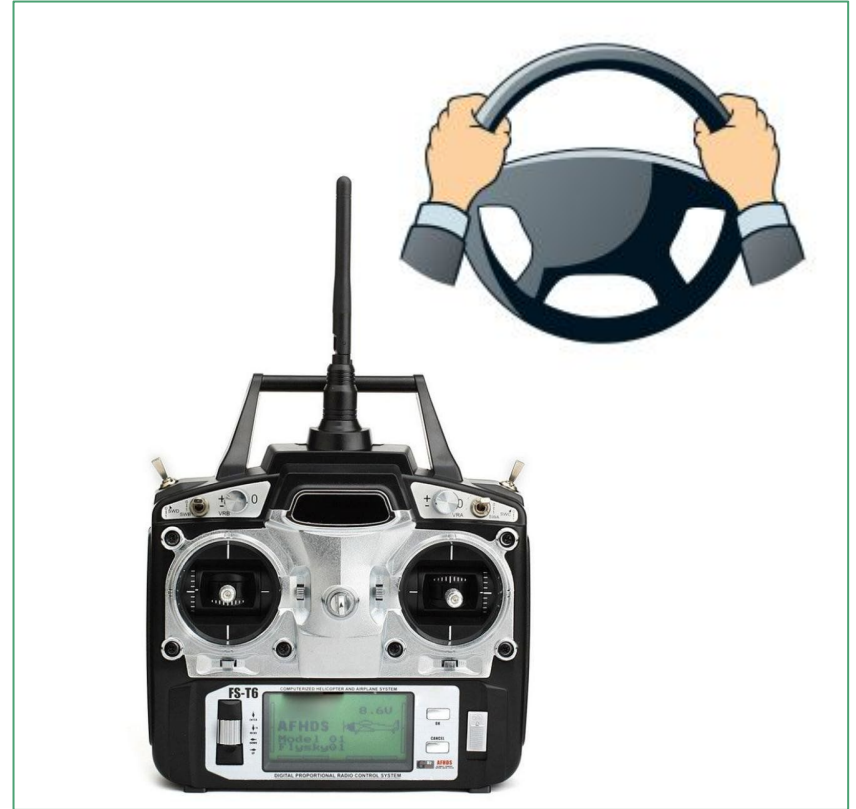
Figure 13: RC Transmitter for control of the Robo-Weeder.
