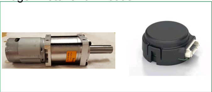
Figure 11: Installation of encoders onto the steering and auger motors.
