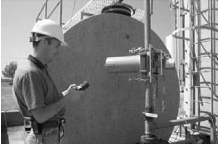
FIGURE 10.3 Nuclear density analyzer (photo published with permission of ThermoMeasureTech, Inc., Waltham, Massachusetts).
