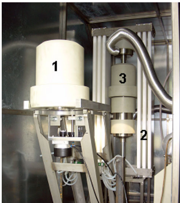
Fig. 10 Batch-processing of green biomass: Hydraulic press and automated feeding system; 1: Test vessel on feeding system; 2: hydraulic press; 3: Test vessel inserted into press during processing
