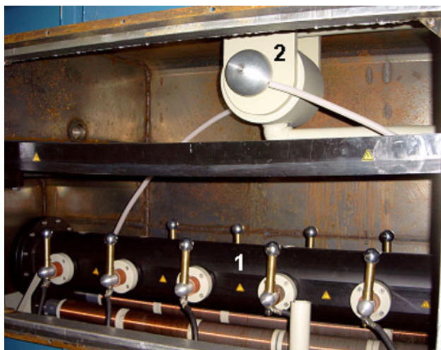
Fig. 13 Electroporation reactor for grape mash: 1: Marx generator; 2: Electroporation reactor
