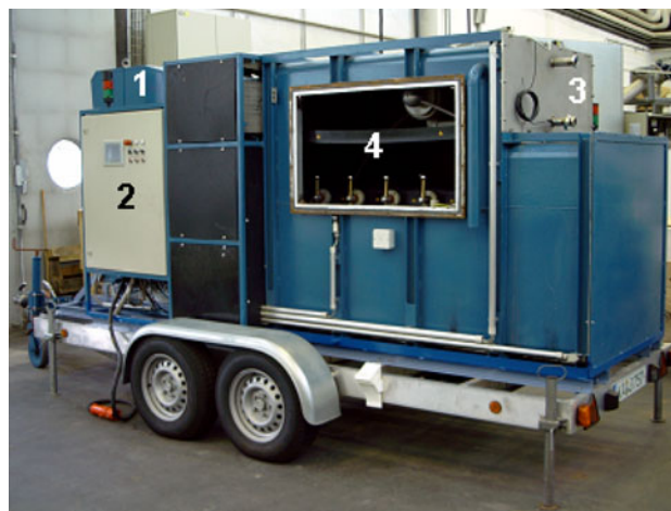
Fig. 11 Electroporation device for grape mash: 1: High-voltage power supply; 2: Control unit; 3: Inlet and outlet for mash (with tubes disconnected); 4: Marx generator and electroporation reactor (details see Fig. 13)
