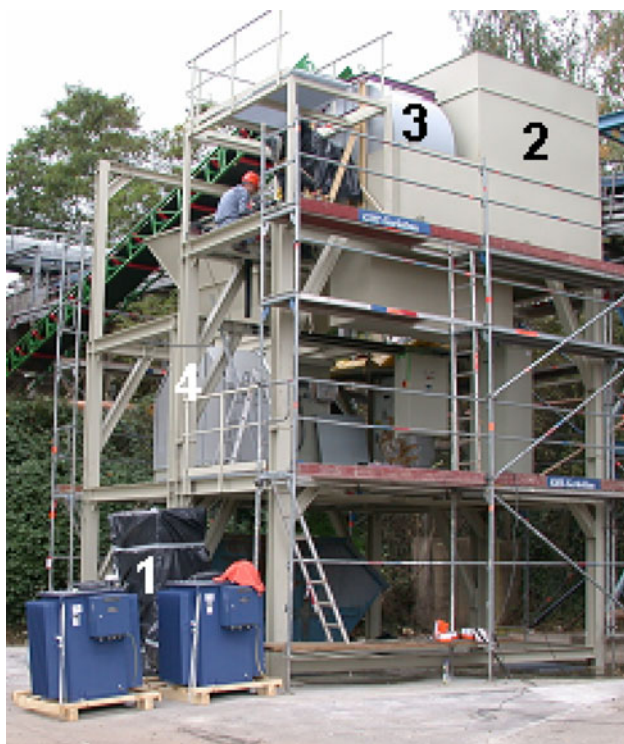
Fig. 14 Electroporation-device for whole sugar beets. The photograph has been taken during construction of the device. 1: Power supplies; 2: Shielding cabin for Marx generators; 3: Electroporation reactor (details see Figs. 15, 16); 4: Slicing machine
