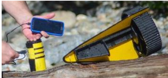
Figure 1 - StreamBee, powers small electronic devices with a USB port
