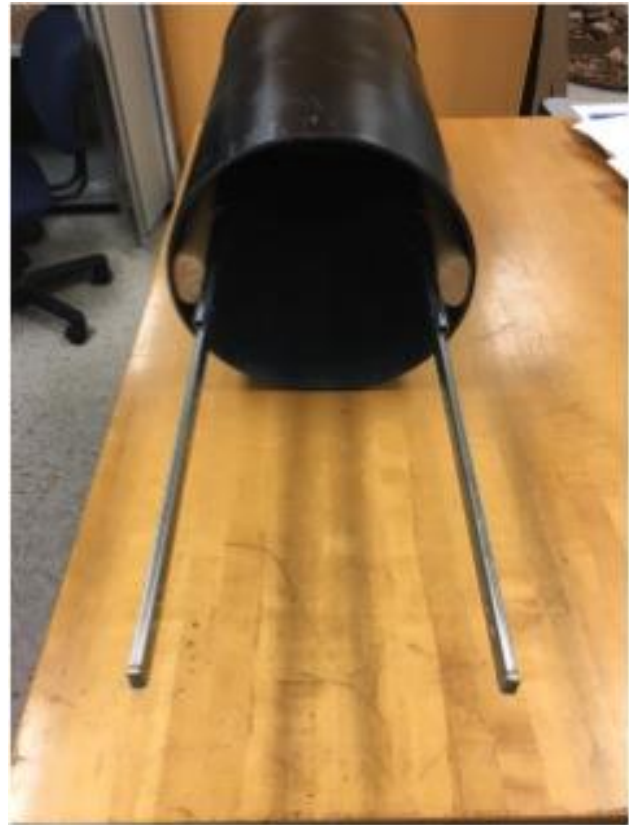
Figure 5: Housing assembly with sliding rails
