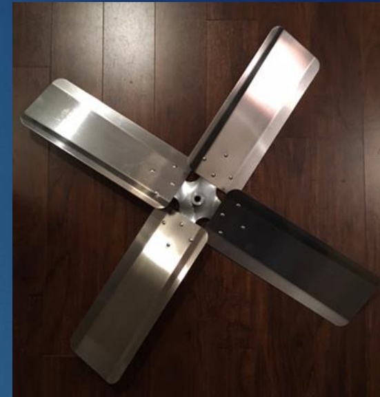
Fig. 6 - 3 ft. Diameter Aluminum Turbine
