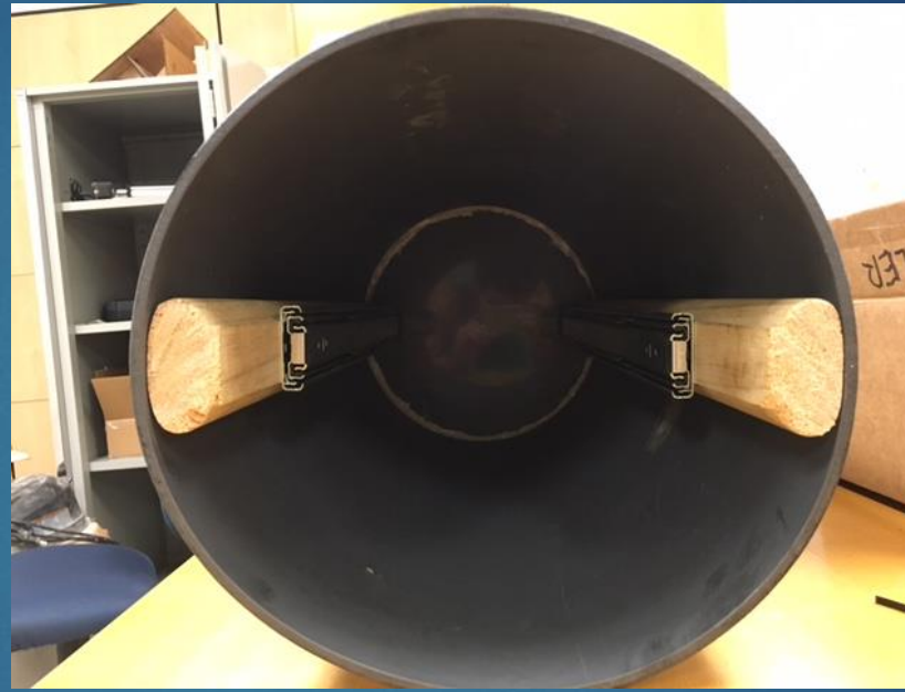
Fig. 13 – Inside of outer PVC housing and railing
