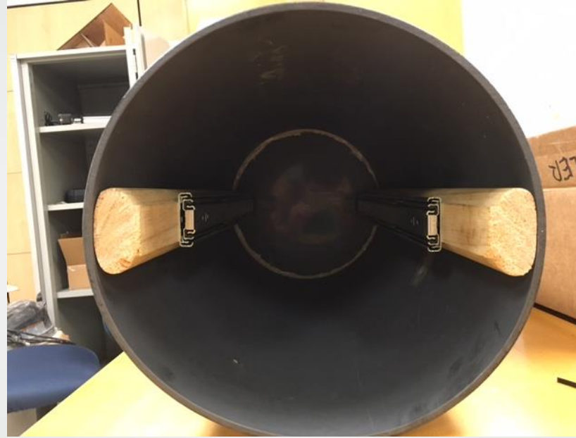
Fig. 14 – Inside of outer PVC housing and railing
