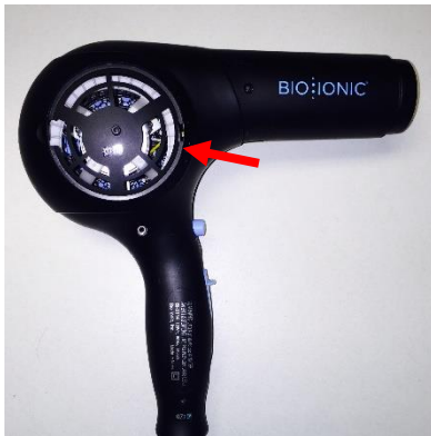
Intake baffle removed from flow path
