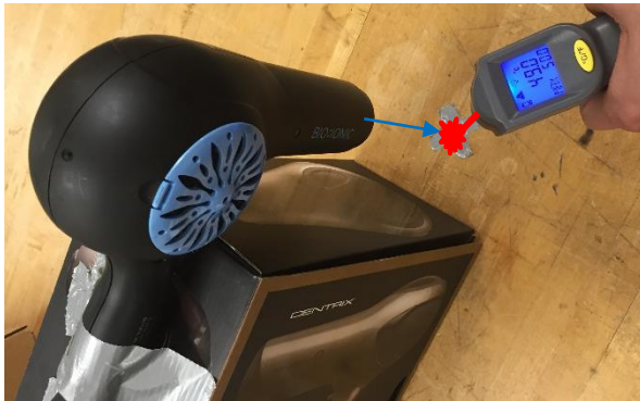
Temperature measurements w/ infrared thermometer
