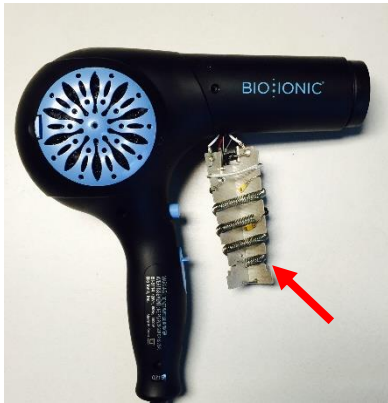
Heating element removed from flow path
