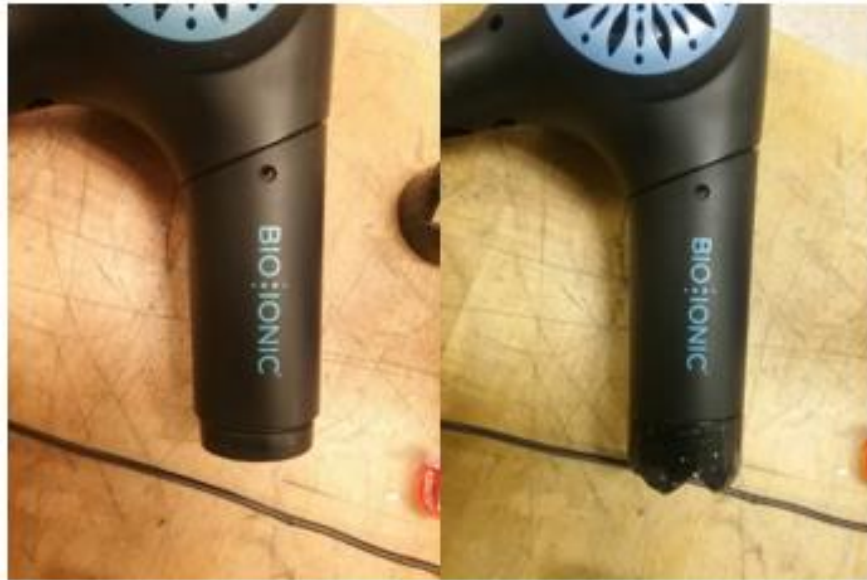
Figure 13: Chevron Nozzle applied to Whisper, before and after
