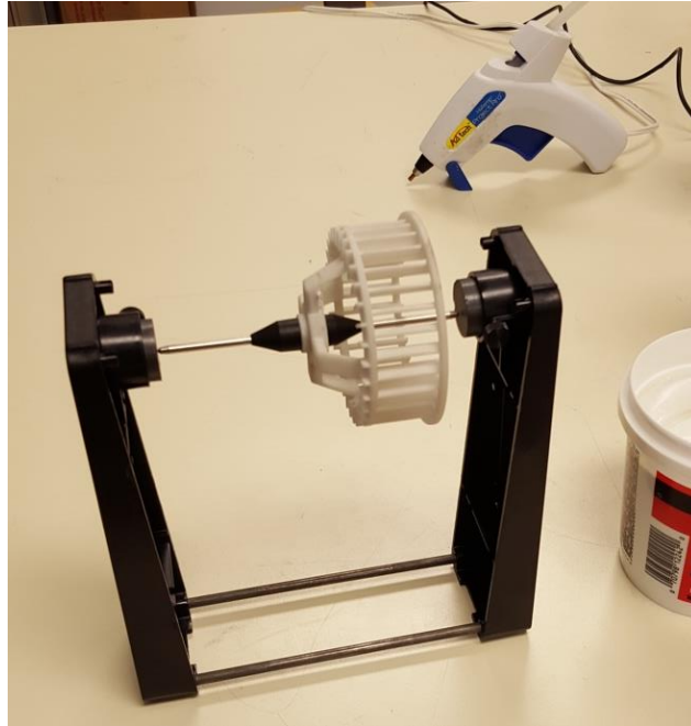
Figure 21: Static fan balancing on a prop balancer
