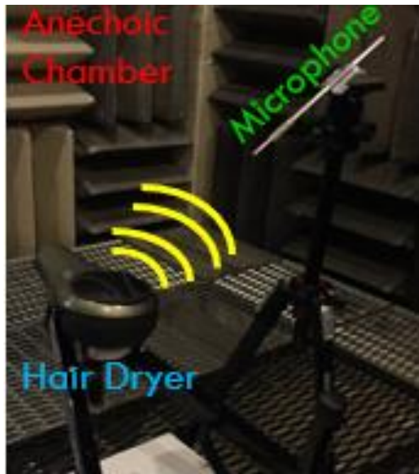
Figure 6: Sound-testing setup in the anechoic chamber
