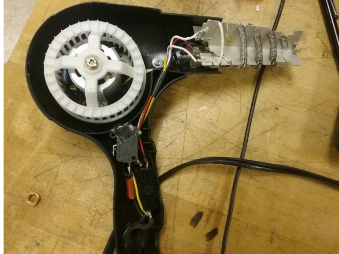
Figure 3: Inside of centrifugal-type hairdryer
