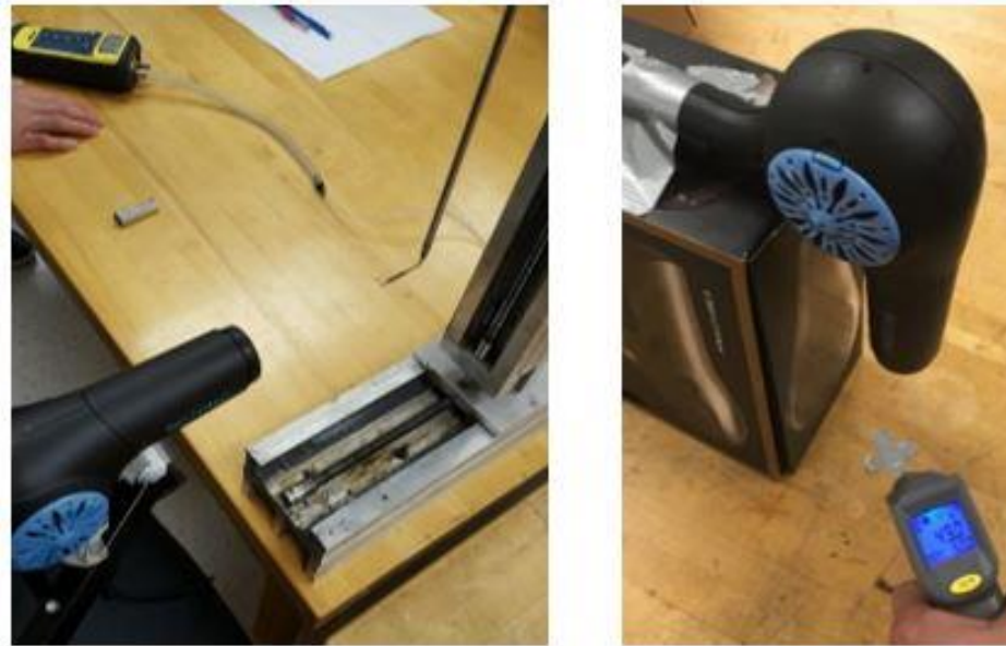
Figure 5: Pitot tube measuring total pressure of hairdryer jet (left) and an infrared thermometer measuring temperature change of the surface (right)
