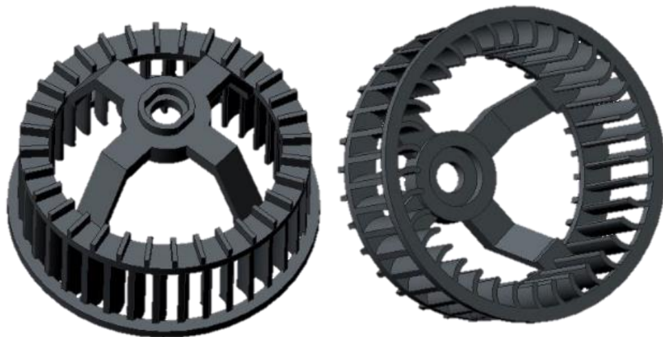
Figure 15: Original Fan recreated in SolidWorks
