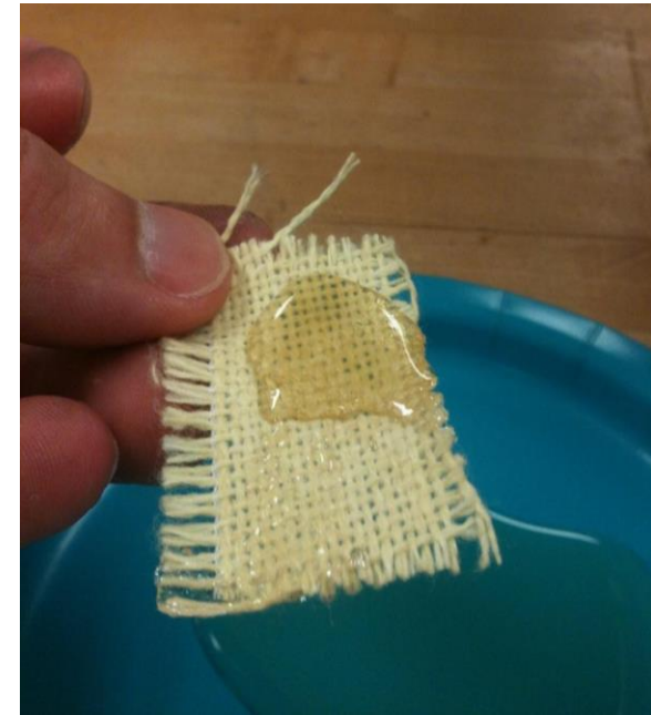
Figure 23. Fiber cloth material after impregnation and oil droplet dispersed
