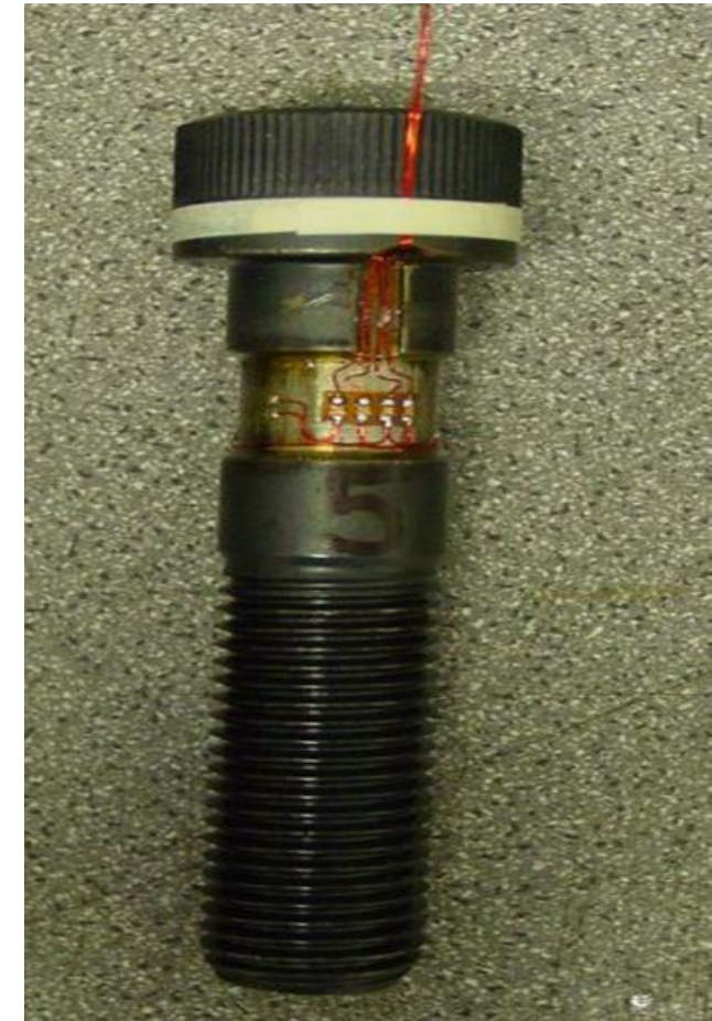
Figure 7. Modified strain gauge bolt
