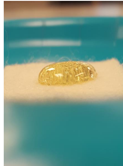
Figure 19. Fiber felt after impregnation and oil droplet dispersed
