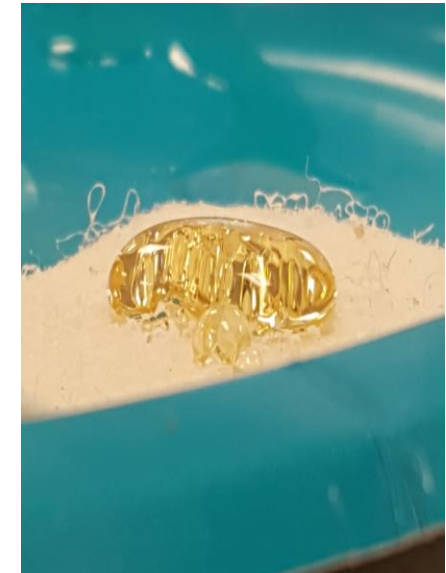
Figure 20. Fiber felt after spray application and oil droplet dispersed
