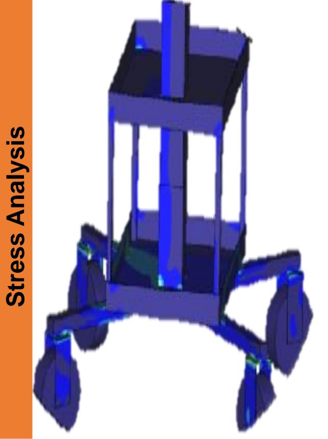
Type: Von Mises Stress Diagram
