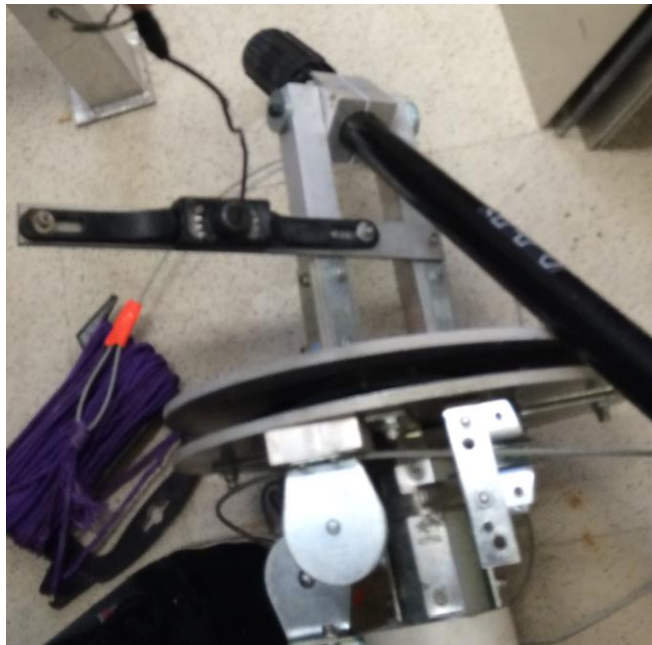
Figure 25 Lazy Susan mechanism
