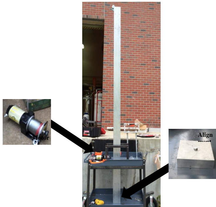
Figure 21. Motor and largest pole mounted on the cart
