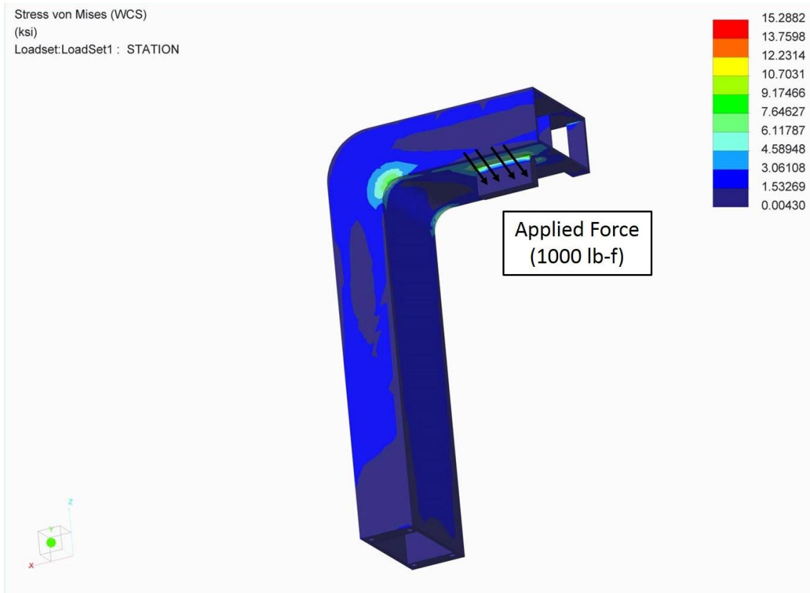
Figure 2.3.2: Structural Stress (von Mises) Back Side
